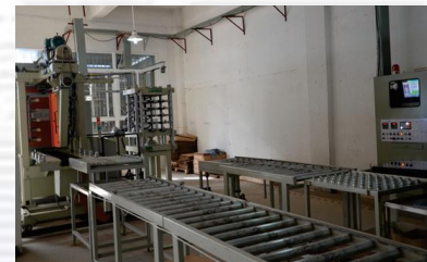
PCB Lamination Line
